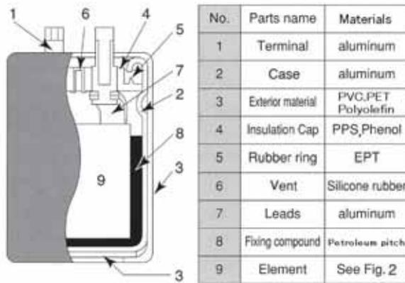
Fig.1 Diagram of Internal Structure (Screw terminal type)
