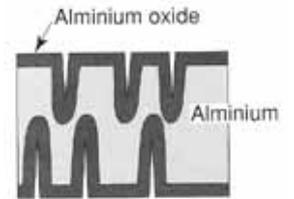
Fig. 4 Diagram of formation model
