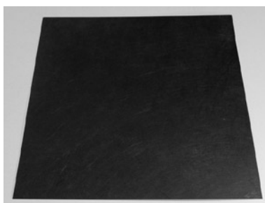
Figure 6 Recycled CFRP using recovered CF non-woven fabric
