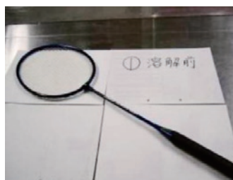
Figure 2 A treated CFRP badminton racket, before (left) and after (right)
