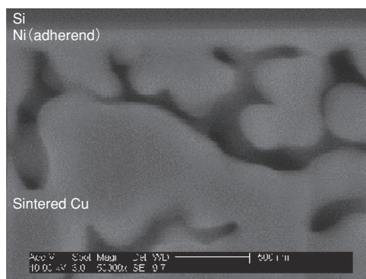
Cross sectional SEM of the bonding interface
