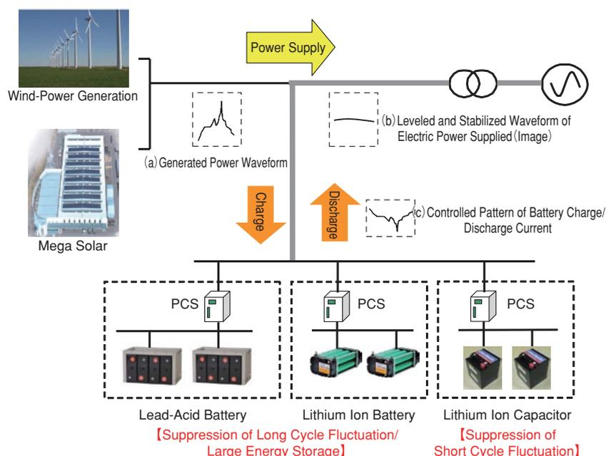
Figure 2 Scheme for Renewable Energy Generation Systems with Hybridized Large Energy Storage Devices
